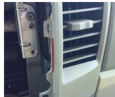
**Area to cut/file out to make InDash and bezel to fit together
