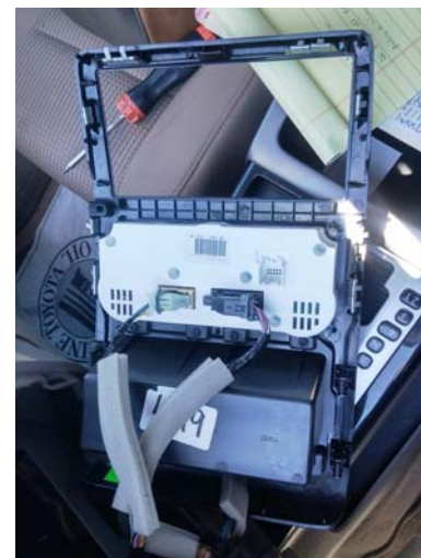
Model Year 13-15 bezel removed, see clips
