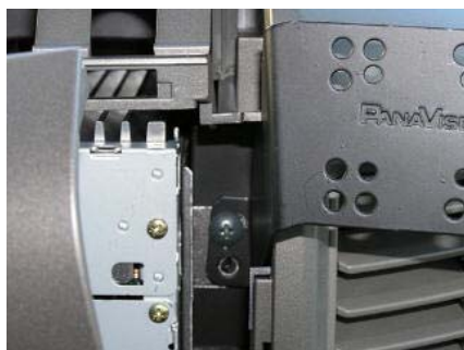
InDash mounted on screw.
